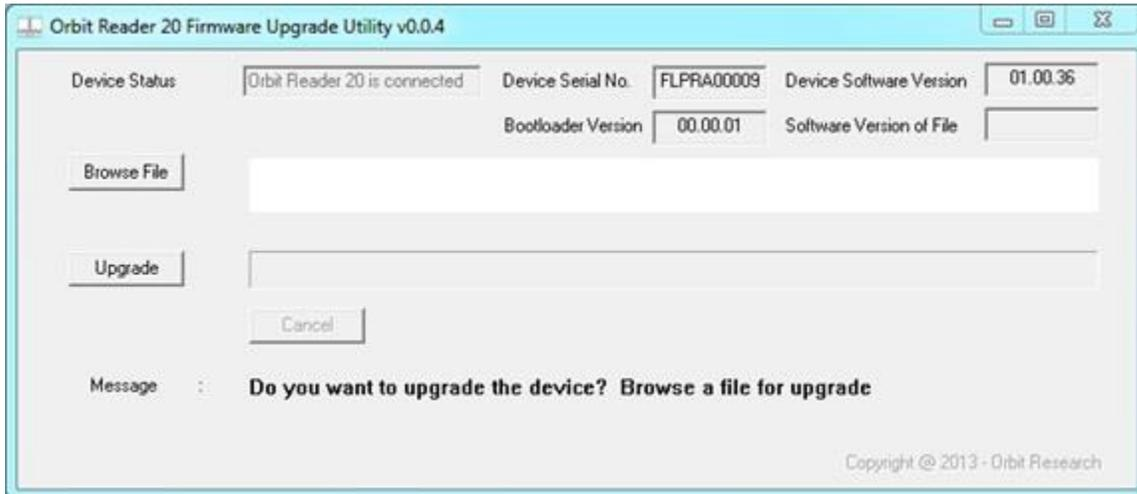
6. The utility shows the device serial number and the software version of the device at top right corner of the window. If the serial number is blank, repeat steps 4 and 5.
