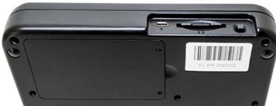
The battery compartment is located on the bottom of the device.
