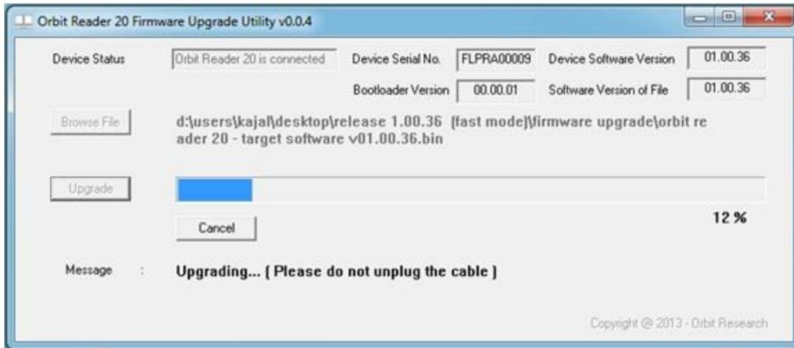
12. Do not unplug the cable. Wait for the message "Device upgrade has been completed" on the upgrade utility or until the Orbit Reader reboots and shuts down.
