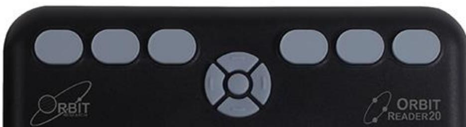
In Stand Alone mode, the braille input keys are the file navigation controls. For example, dots 3 and 6 serve as Page Up and Page Down to move through a title.
